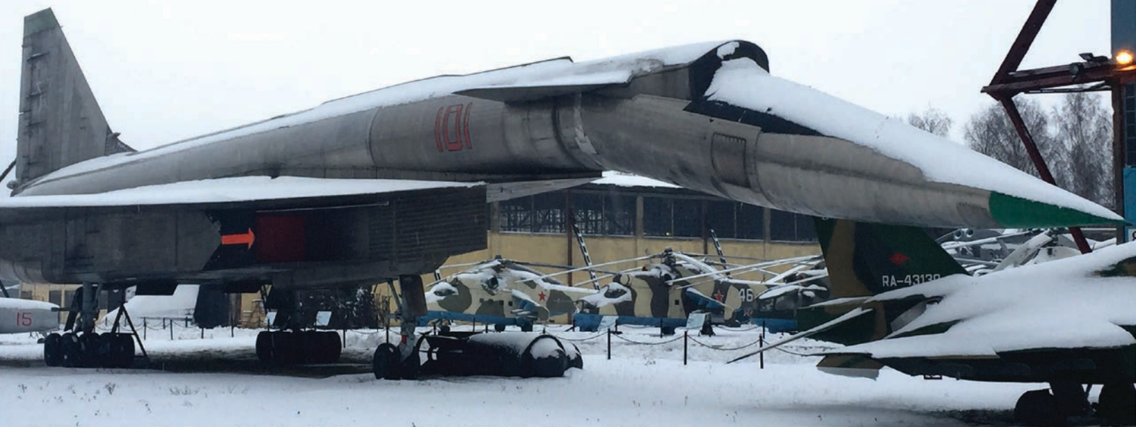
The T-4 experimental supersonic bomber (also known as the Su-100) first flew in August 1972.
